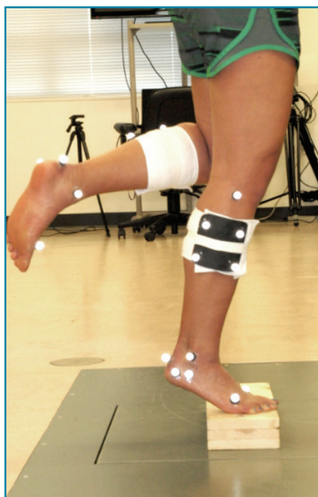
Figure 1. Reflective markers defining the 2-segment biomechanical model of the lower leg and foot.
