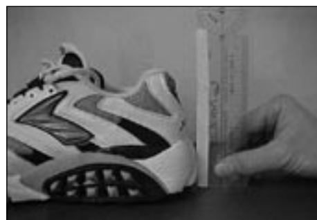
Figure 3. Qualitative assessment of the posterior heel flare for the Brooks Beast (Brooks Sports, Inc.; Bothell, Wash) running shoe. A straightedge is held perpendicular to the support surface against the most posterior aspect of the shoe. Space between the anterior edge of the ruler and the posterior aspect of the heel counter is noted.
