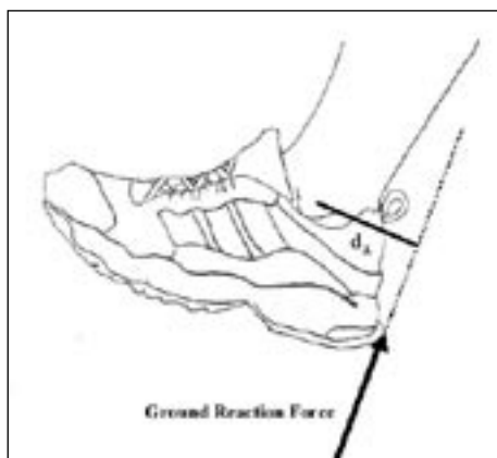
Figure 2. Positive posterior flare tends to increase the moment arm distance ( d_1 ) between the ground reaction force and the ankle joint at heel strike.
