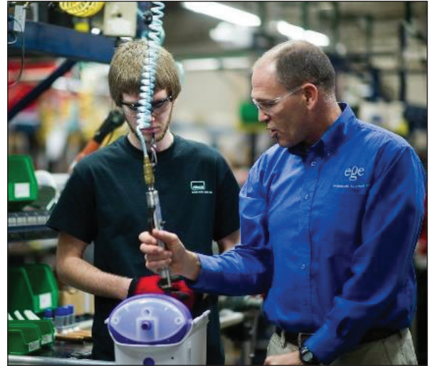
Figure 1. Example of Job Coaching for Use of an Inline Power Tool Using Neutral Wrist Positioning
