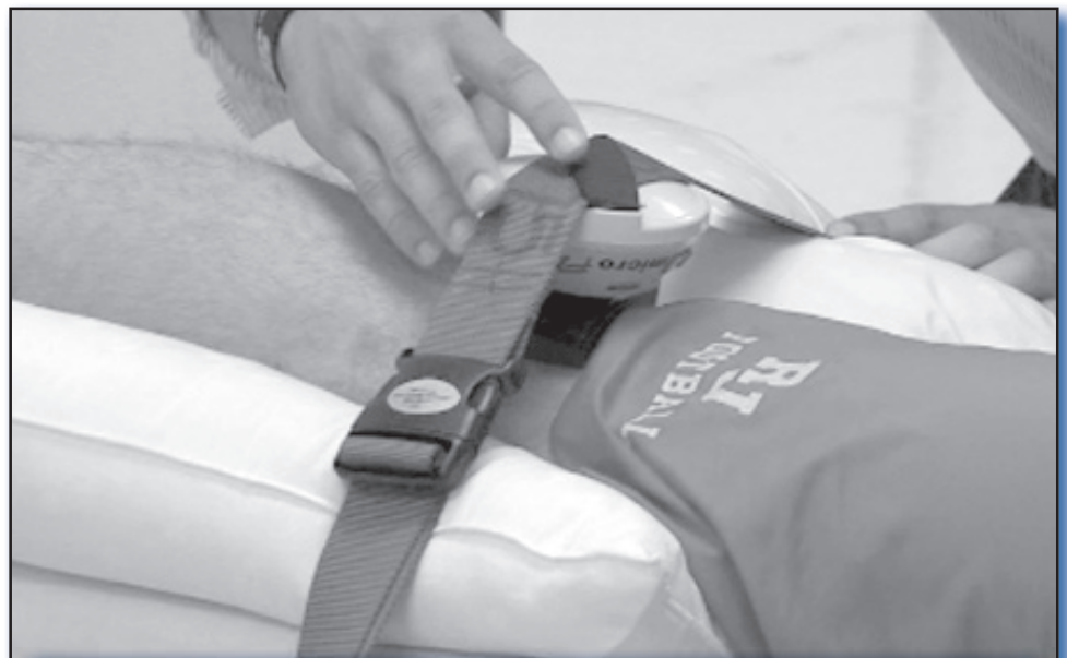
Figure 9. Placement of dynamometer to assess hip abduction strength.
