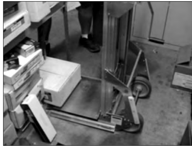
Step 4. Remove tire to be rotated to open hub position.
