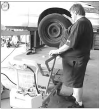
Step 3. Manipulate tire in mid-range to horizontal position on back of cart.
