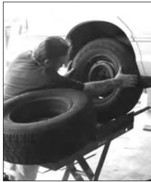
Step 4. Remove tire to be rotated to open hub position.
