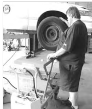
Step 2. Operate battery-powered lift cart to remove tire from car.
