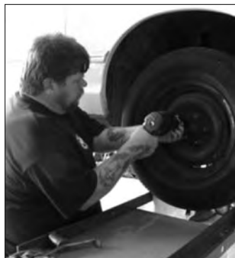
Step 1. Operate small impact wrench to loosen and remove lug nuts.
